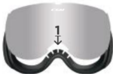
Connect the joints of the lens to the frame, start from the joints placed up to the nose pad (the joints are highlighted in figure with number 1).
